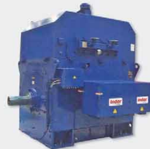
Asynchronous motor, to drive the discharge pump to the land
